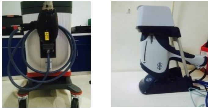
Photo 8: Non-intrusive instruments: handheld XRF & Mobile OES
