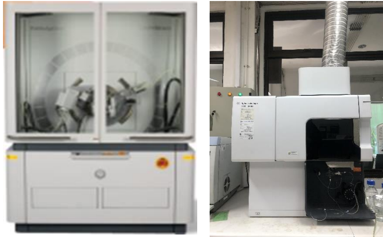
Photo 4: Analytical instruments for mineral analysis: XRD & ICP-OES
