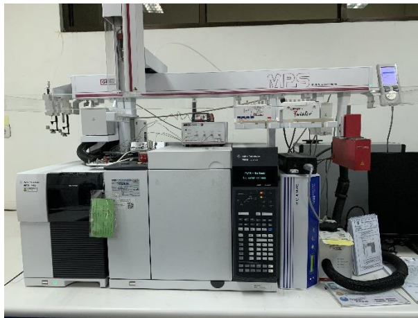
Photo 5: GC-MS with multi-purpose autosampler
