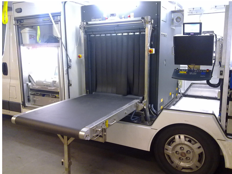
Interior of the Mobile X-ray with conveyor deployed
