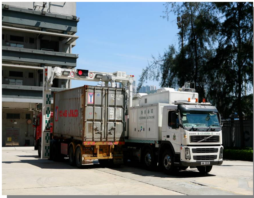
A Mobile X-ray Vehicle Scanning System scanned a container truck at Kwai Chung Customhouse, Hong Kong
