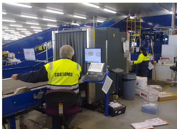
Example of a Smiths 100x100 Cabinet X-ray
