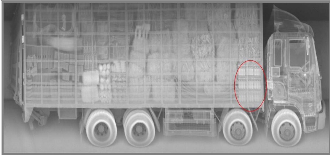
Bottles of liquor mixed with general cargoes are revealed by a backscatter X-ray scan
