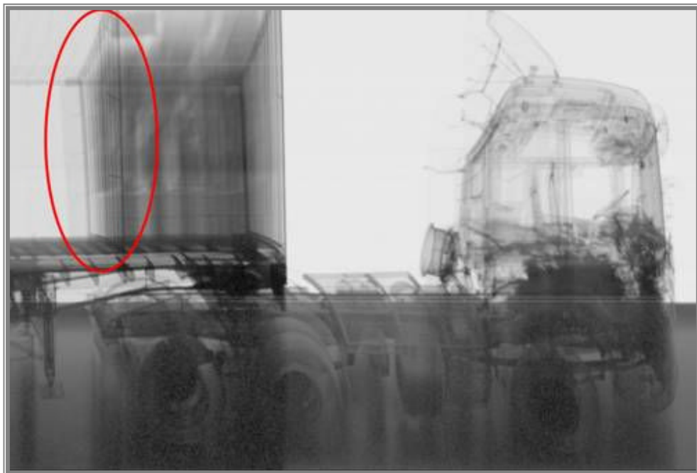
Cartons of cigarette concealed in a false compartment of a container truck are revealed by a transmission X-ray scan
